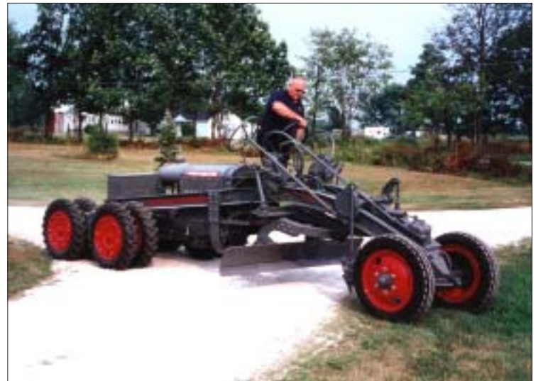
Frank Root, Jr. operating restored McCormick-Deering Warco One-Man Grader (photograph by Lou DeLong).
